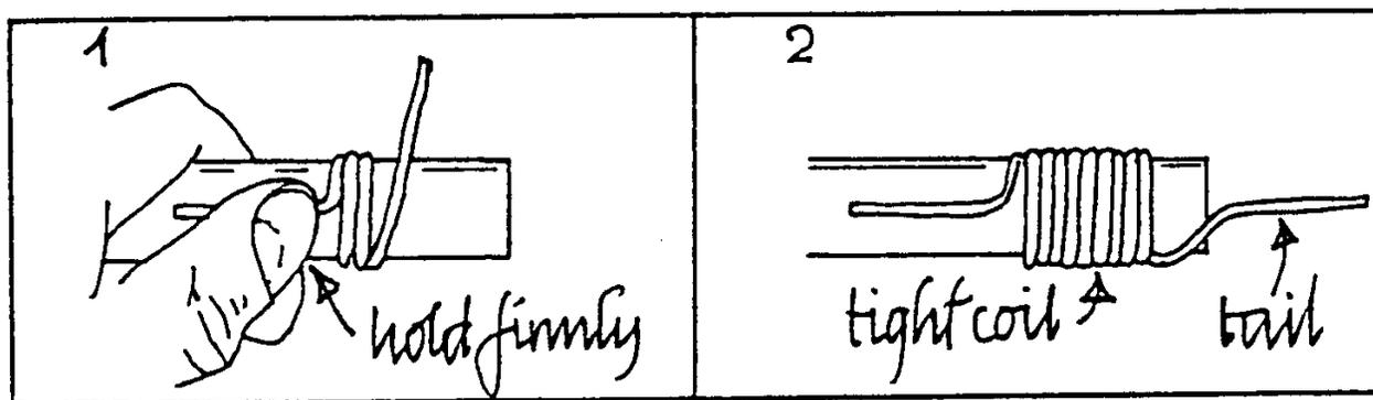
15. Slip the tight coil off the glass tube and adjust the tail so that it bends and then is positioned down the axis of the coil.
