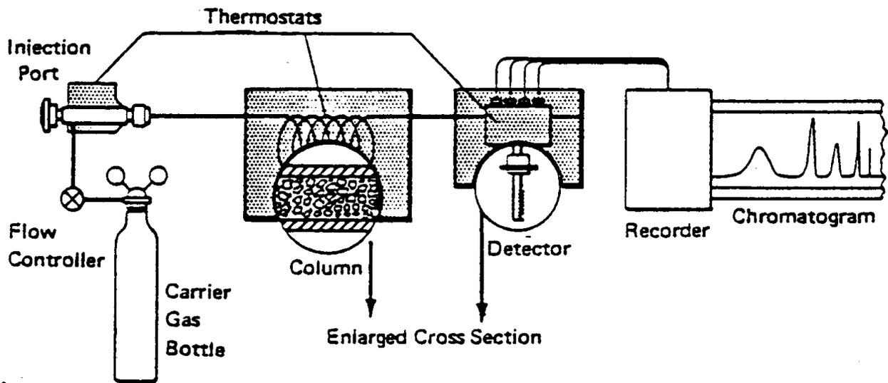
**FIGURE I-1—SCHEMATIC DRAWING OF A GAS CHROMATOGRAPHIC SYSTEM**
