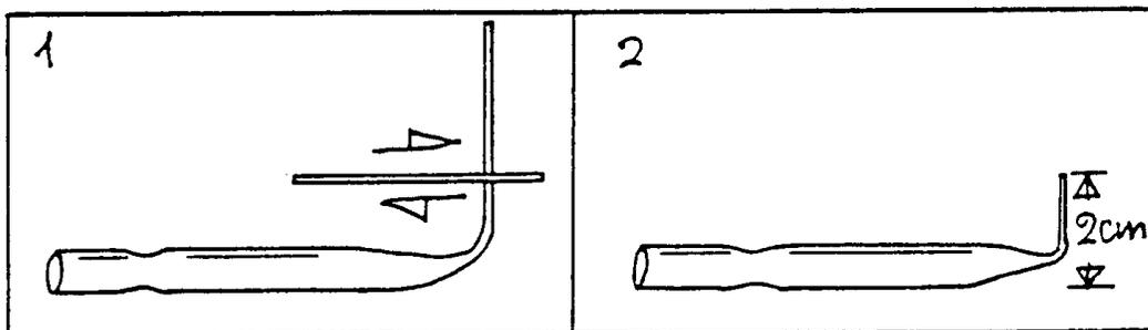
12. Similarly, cut off the larger diameter end about an inch (2-3 cm) from the bend with a scorer or file. Save the cutoff part.
